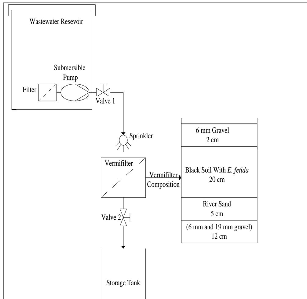
**Figure 1.** Schematic diagram of the vermifiltration system used in all experiments
